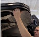
1. If needed, gain access to the underside of the boat in your proposed mounting location. (Remove or lower splash pans or drill a 2 1/2"access hole.)
