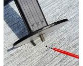
3. Once placement is confirmed, lightly mark the mounting location on the flooring surface.
