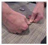
5. Push the Ghost Mount body into the mounting location. (If your mounting location is close to a cross-member, confirm the proper positioning of the "flats" on the mounting body in relation to the stamped retaining washer that will be placed on the bottom side.)
