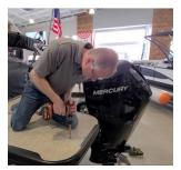
4. Using a very sharp drill bit, drill a 5/8" hole, straight-down, in the mounting location. Clean up woodchips, above and below deck, to ensure a smooth surface both above and below deck to ensure a clean path for the mounting body.
